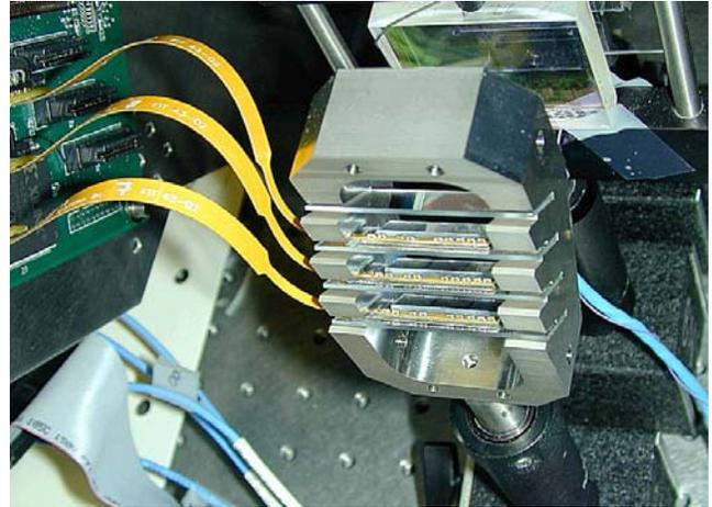
Figure 4. Photograph of 3x3 liquid crystal on silicon optical phased array of phased arrays in housing.
