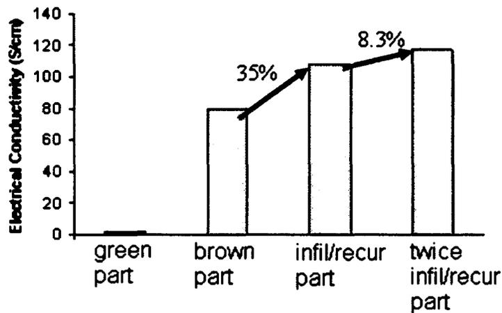
Figure 2. Electrical conductivity improvement of SLS bipolar plate with respect to corresponding fabrication step.
