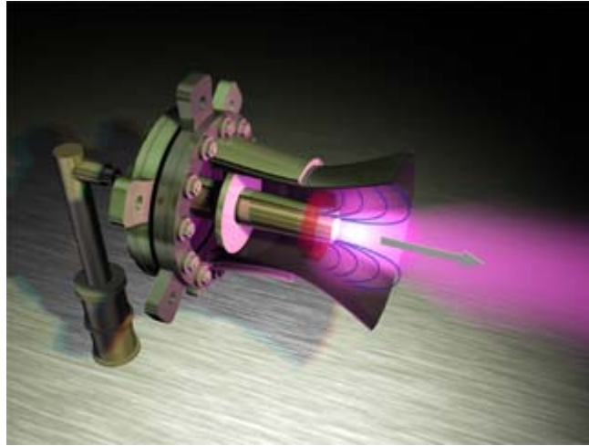
Figure 14: Self-field MPD Thruster
