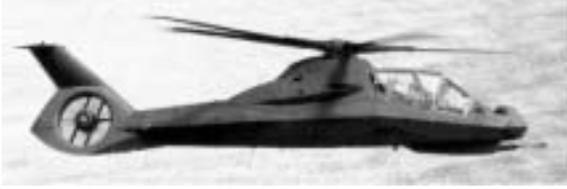
*The new RAH-66 Comanche was the Army's most advanced helicopter and the cornerstone of the Aviation Modernization Program. The aircraft featured "stealth" which had previously been confined to airplanes.*
