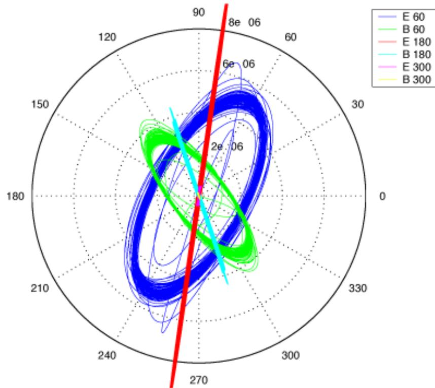
Figure B6: Example of E and B field polarization ellipses at odd harmonics: 60, 180, and 300 Hz.
