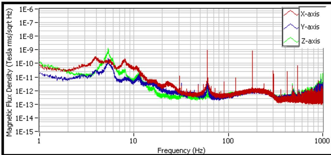
Figure B4: Magnetic induction spectral density display of X, Y, and Z axes from low-frequency sensors. The X-axis is pointing approximately  $-0.15$  degree from magnetic north. The Y-axis is pointing west, and the Z-axis is pointing down.
