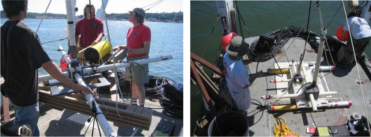
Figure 5: (left panel) E-field system being prepared for deployment. (right panel) B-field instrumentation being assembled prior to deployment on R/V Miller.
