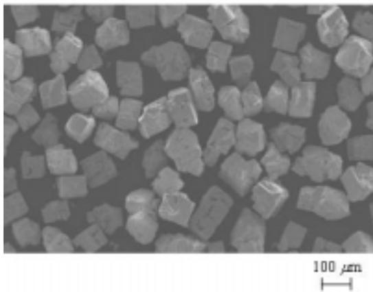
Fig. 2 PZT single crystals obtained by a PbO flux method.
