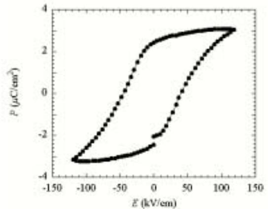
Fig. 5 DE loop of 1-3 composite sheet.
