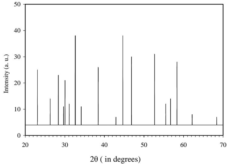
Figure 1. X-ray powder diffraction pattern of  $\text{Sr}_{0.8}\text{Na}_{0.4}\text{Nb}_2\text{O}_6$  ceramics.
