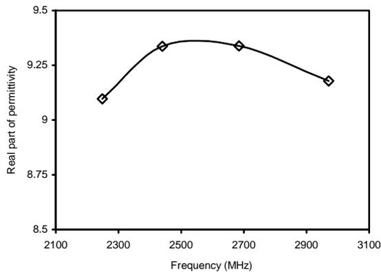
Figure 3. Frequency versus real part of complex Permittivity of SNN ceramics.
