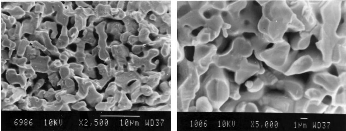
Figure 2 Scanning electron microscope photographs of SNN ceramics.
