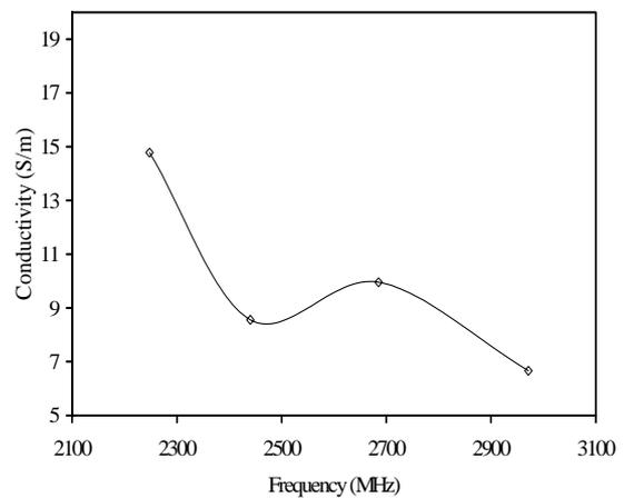
Figure 6. Frequency versus conductivity (S/m) of SNN ceramics.
