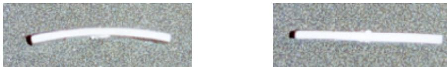
**Fig. 2** Monolithic BTS ceramics sintered with two layers of BTS7.5 and BTS15 (left) and with four layers BTS7.5-BTS10\_BTS12.5-BTS15 (right)
