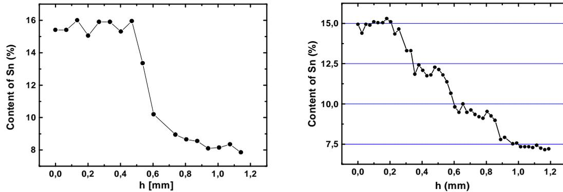
**Fig. 1** Content of tin along the thickness of monolithic ceramic samples sintered with two (left) and four layers (right) of BTS
