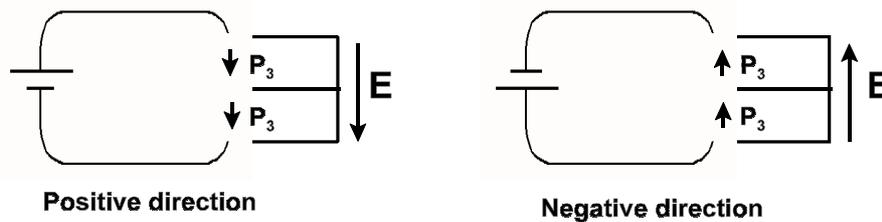
**Fig. 5** Definition of the poling direction of the BTS7.5-BTS15 system
