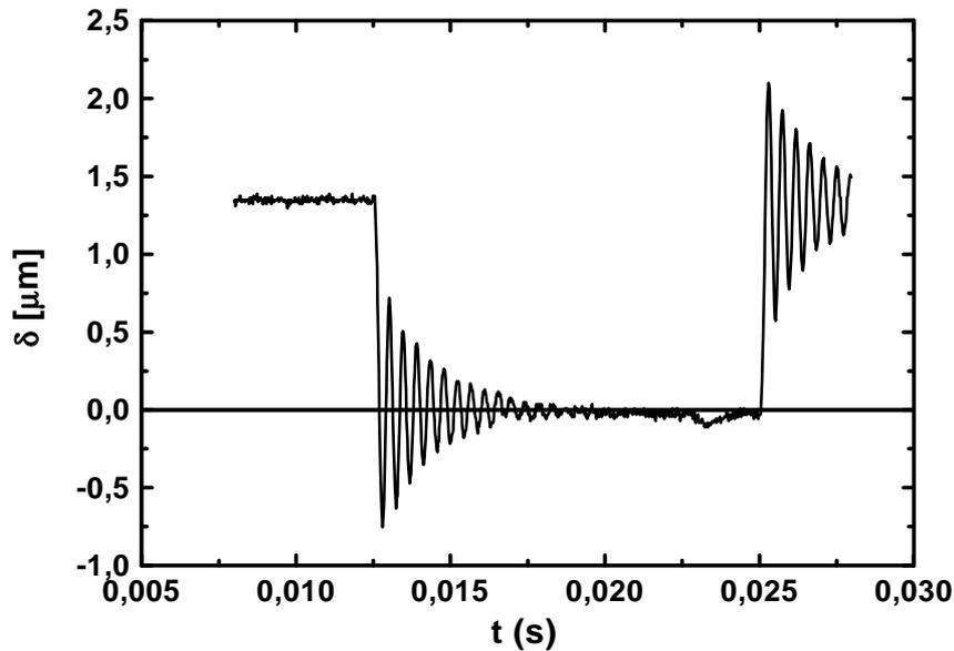
**Fig. 10** Free vibration response of a one side fixed monolithic FGM actuator
