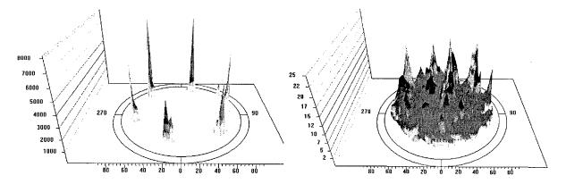
Figure 2a: (1123) pole figure of the Al<sub>2</sub>O<sub>3</sub> phase in an Figure 2b: (311) pole figure of the ZrO<sub>2</sub> phase in Al<sub>2</sub>O<sub>3</sub>-ZrO<sub>2</sub> DSE. Since the phase is nearly single an Al<sub>2</sub>O<sub>3</sub>-ZrO<sub>2</sub> DSE. crystalline, a rotated single crystal stiffness tensor can polycrystalline yet textured, a weighted stiffness be used.
