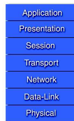
Figure 4: The OSI Idealized Network Model Layers.
