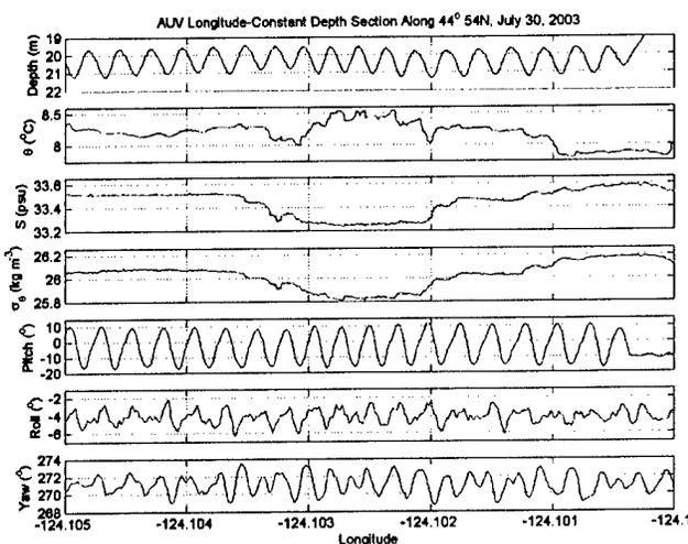
**Figure 3.** A short (~ 400 m) section of small amplitude sawtooth sampling at around 20m depth, showing (from top to bottom): depth of the AUV, temperature ( $\theta$ ), salinity (S), and density ( $\sigma_\theta$ ) along the AUV path, followed by AUV pitch, roll, and yaw. Note that the vehicle pitch changes smoothly as the AUV progresses, and that roll and yaw fluctuations are small amplitude.
