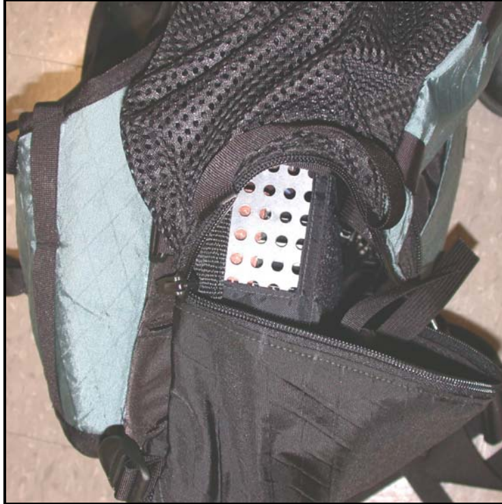
Figure 17. Photograph of the lower side of the backpack showing the vents for airflow in the high voltage pulser box. The side of the backpack is also ventilated and covers the box when in use.
