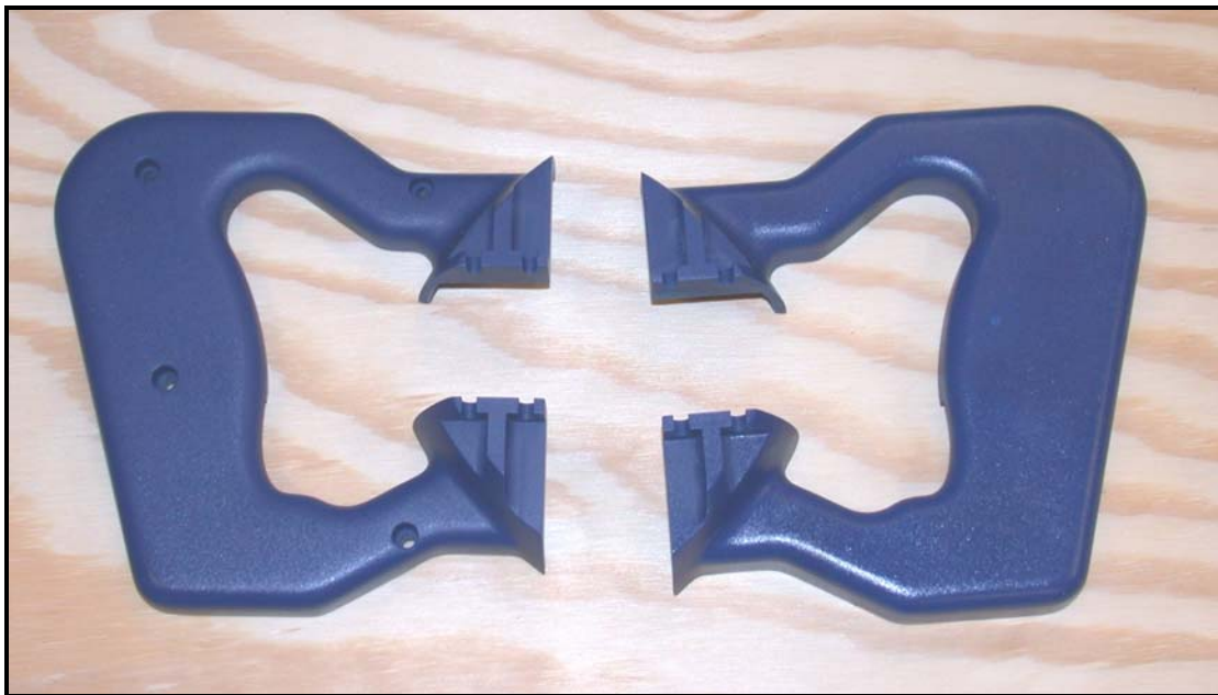
Figure 15. Photograph of the two plastic pieces that form the handle for the TWS sensor and contain the trigger activated switch assembly.
