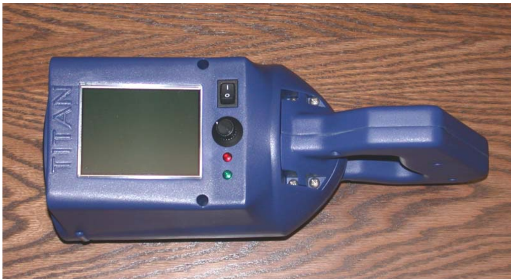
Figure 8. Photograph of the hand-held TWS sensor assembly showing the video display screen, threshold control knob, power switch and indicators.
