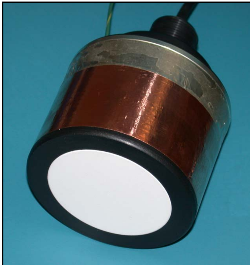
Figure 4. Commercially available Airmar AR-41 transducer with Jaycor’s custom circumferential copper ground shield for low noise operation.
