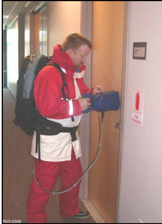
Figure 2. Photograph of TWS prototype system being demonstrated on a solid wood door.
