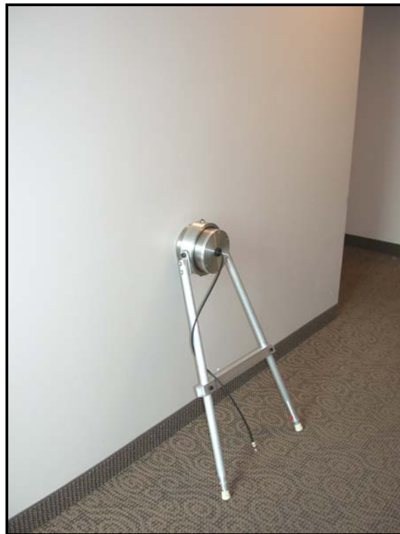
Figure 21. Photograph of the stand-alone mounting fixture designed to apply a uniform force on the transducer/wall interface.
