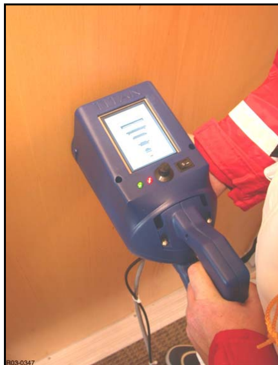
Figure 3. Close-up photograph of the prototype handheld display unit during operation.
