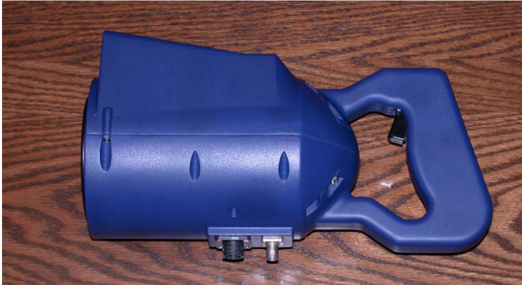
Figure 9. Side-view of the TWS hand-held assembly showing the cable connections on the bottom for the high voltage pulse signal, video, and power feeds.
