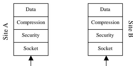
Fig. 1. Architecture of the data exchange service
