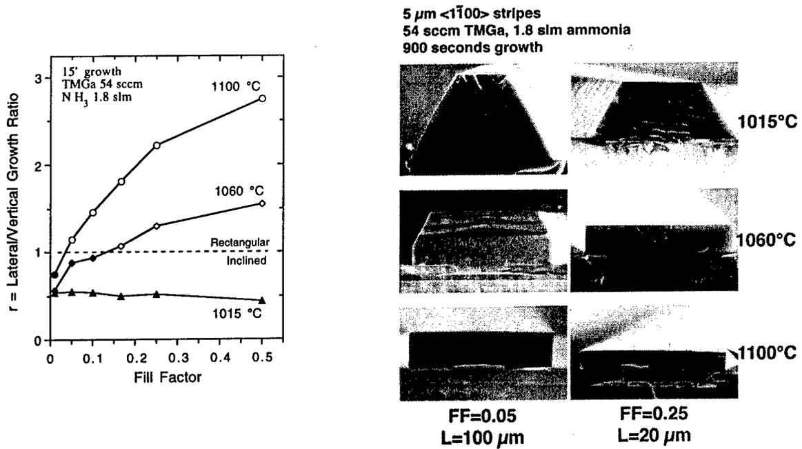
Figure 6. Effect of temperature on (a) lateral-to-vertical growth ratio and (b) LEO morphology.
