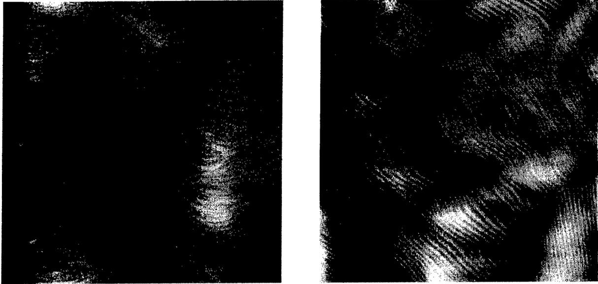
Figure 8. AFM images of (a) bulk GaN and (b) LEO GaN surfaces. Threading dislocations appear as small black pits. Note the step arrays on the LEO GaN surface. Image size is  $8 \times 8 \mu\text{m}$  in both cases.
