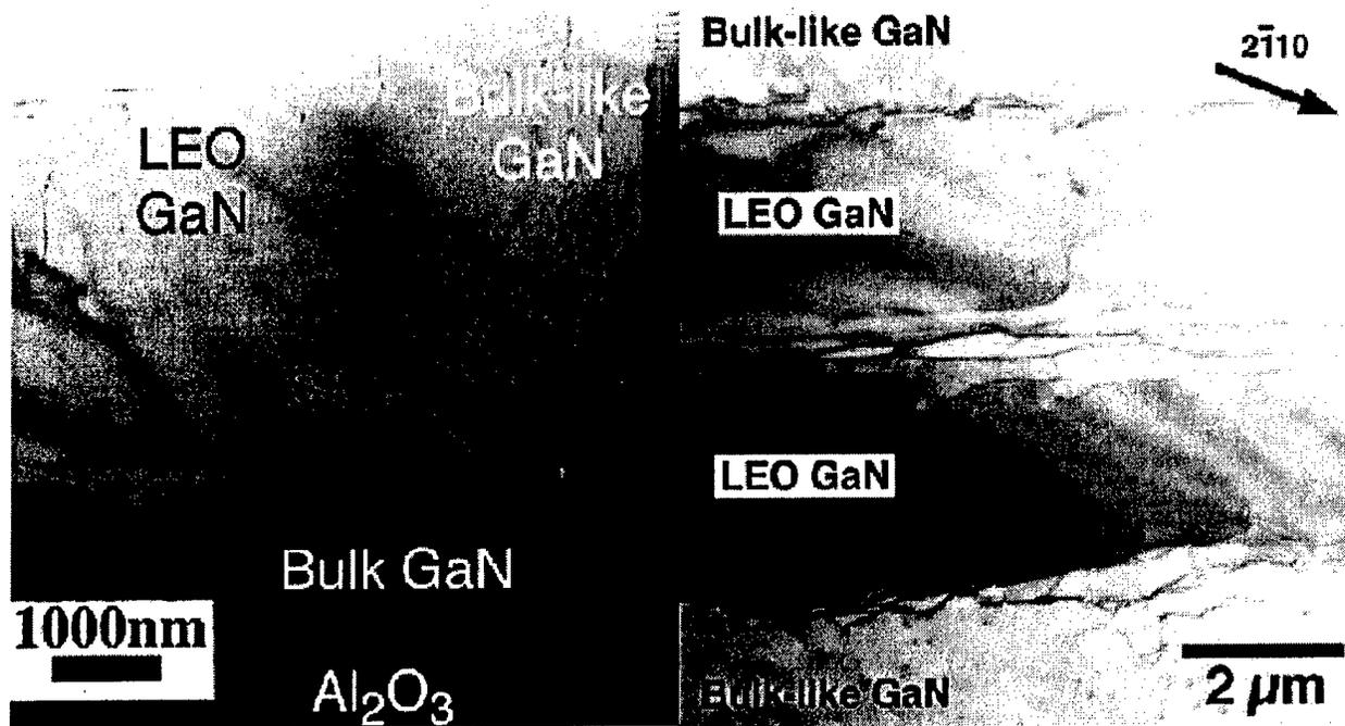
Figure 7. Cross-section transmission electron micrograph of LEO GaN stripe. Note near absence of dislocations in the LEO region above the SiO<sub>2</sub> mask compared to the bulk GaN regions. (b) Plan view of coalesced LEO film. Note dislocations lying in the plane of the film near the LEO/bulk interface and at the intersection between adjacent LEO stripes.
