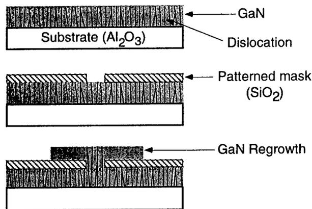
Figure 1. Schematic of lateral epitaxial overgrowth (LEO) technique.
