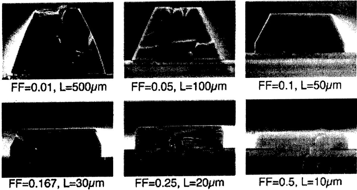
Figure 5. Cross-sectional SEM images showing effect of fill factor on LEO GaN morphology. Note the gradual trend from inclined to vertical sidewalls with increasing fill factor.
