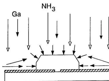
Fig. 4(a) Plot of net volume of growth as a function of mask stripe fill factor. (b) Schematic representation of enhanced supply of Ga from the mask regions that leads to a fill factor-dependent local V/III ratio at the growth front.
