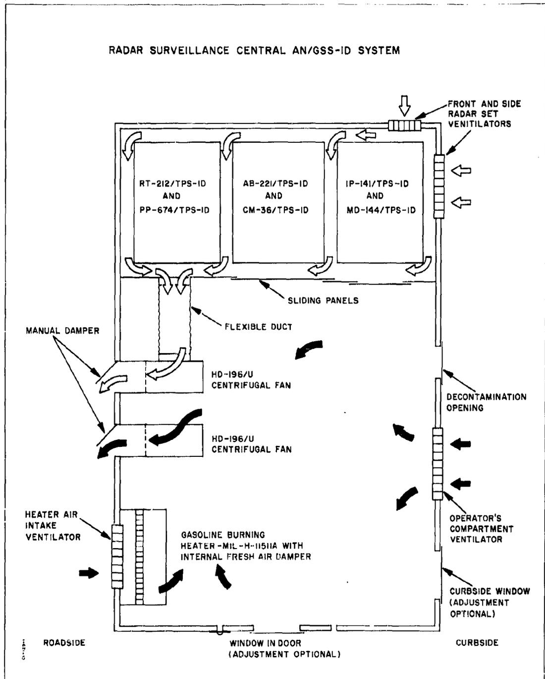
Figure 1 Equipment Compartment: Cooled by Ambient Air
