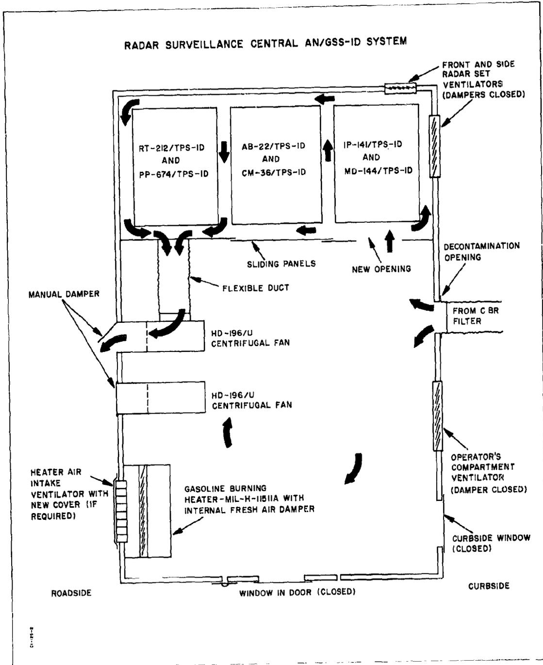
Figure 2 Equipment Compartment: Cooled by CBR Air
