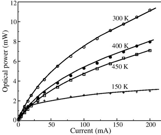
**Fig. 1.** Light-current characteristics of green Nichia InGaN SQW LED in temperature range up to 450 K. Curves are calculated with recombination coefficients as fitting parameters. Diode area is  $7 \times 10^{-4} \text{ cm}^2$ .
