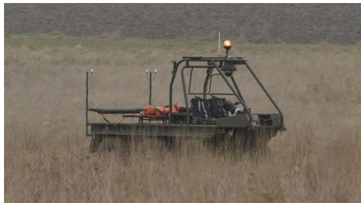
Figure 5 BAE systems Multi-Operated All-Terrain Vehicle has been developed to remotely supply and support troops in the field [35].
