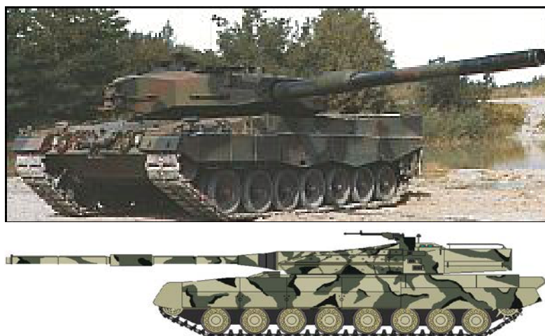
Figure 3 In 1983 fear of new soviet tanks led Germany, the Netherlands and Switzerland to commence experimentation which led, by the early 1990's, to this concept demonstrator of a 140mm gun on the Leopard 2 (top). At the time, rumours abounded about 135mm or 152mm (bottom) Soviet tanks ... but there were only ever drawings of what the West thought the Soviets may have.
