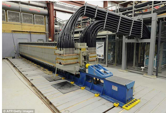
Figure 4 The US Navy Electromagnetic Cannon (rail gun) successfully test fired in December 2010[33].
