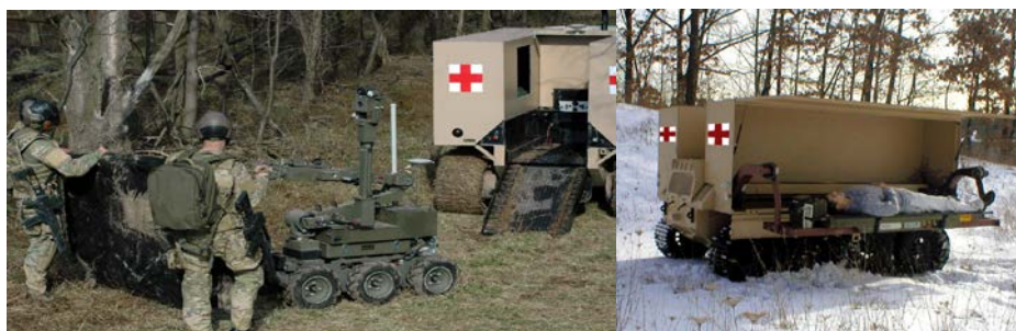
Figure 7 Robotic Evacuation & Extraction Vehicles being developed for the US Army Medical Robotics Research through the Army's SBIR (Small Business Innovation Research) Program [36].
