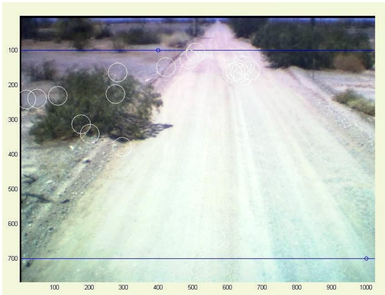
Figure 3: One frame of a typical video image sequence. The faint white circles indicate potential target hits in this video frame.
