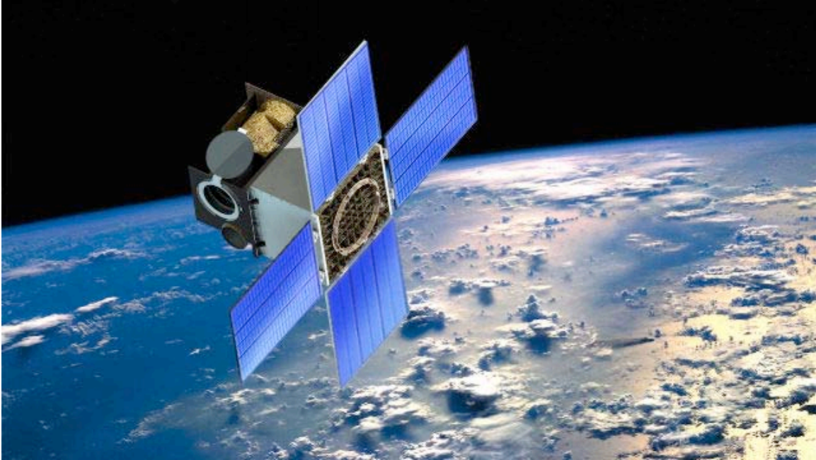
Figure 1. Current JMAPS spacecraft concept. Primary instrument is an 8” visible/near IR telescope. Spacecraft is microsat-class.
