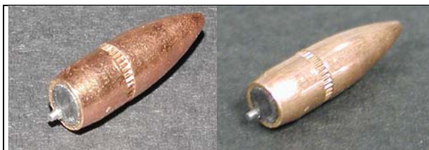
Figure 4. Pristine (left) and pre-engraved (right) 5.56 mm projectiles
