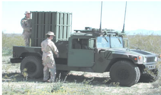
Figure 6. NLOS-LS Box Containing 16 Slots
