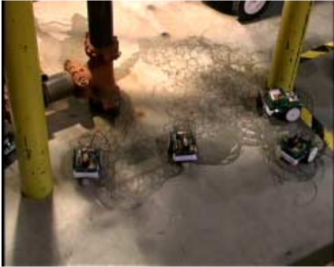
Figure 9: Robots deployed in a cluttered DOE facility form a perimeter around a water spill.
