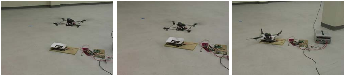
Figure 7: Fully Autonomous Landing and Recharge Demonstration
