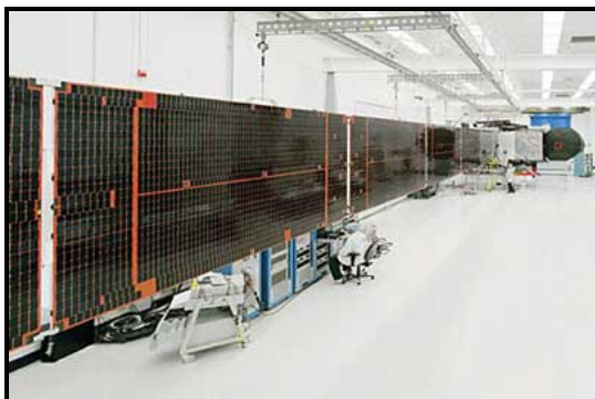
Figure 4 – Rigid Panel Array
