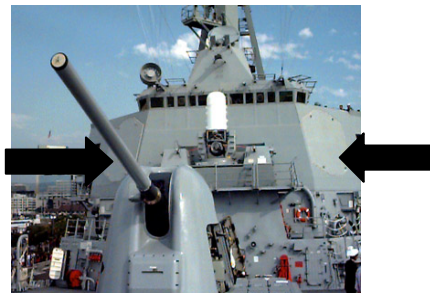
Figure 3. Spy-1D Phased-array Radar Antennas (2 of 4 shown) (Source: After Global Security.org, 2006)
