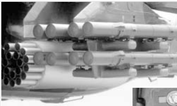
Close-up views of Mi-28 Havoc systems at a Paris International Air and Space Show, Le Bourget Airfield. (Left) Rockets and missiles include the laser-guided Vikhr with a proximity fuse for use against helicopters. (Below left) The Havoc's laser target indicator allows for rapid engagement and disengagement.
