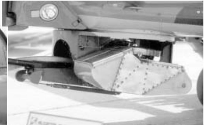
(Above) The Mi-28's stabilized 2A42 cannon can effectively fire an exploding 30-mm fragmentary round with proximity fuse out to 4,000 meters. The 30-mm cannon and Vikhr missile system are well suited to helicopter v. helicopter operations.
