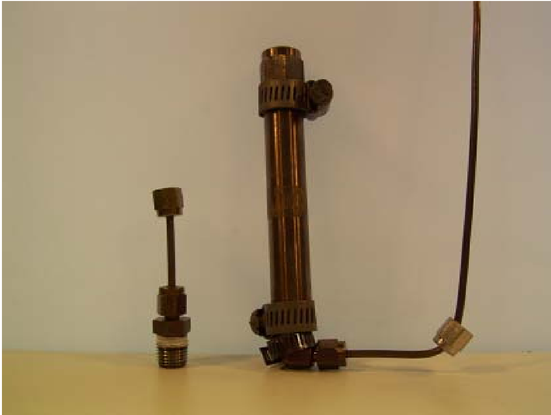
Figure 2. Gravimetric JFTOT vessel. Note the discolouration of the stainless steel which has been caused by exposure of the vessel to high temperatures in the sand bath.
