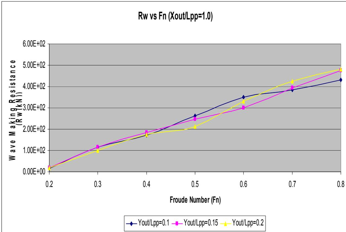
Figure 27. Wave Making Resistance Results for  $X_{out} / L_{pp} = 1.0$
