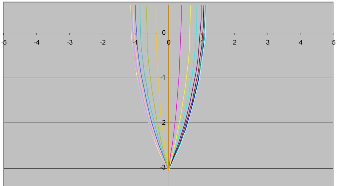
Figure 6. Body Plan of the Side Hull
