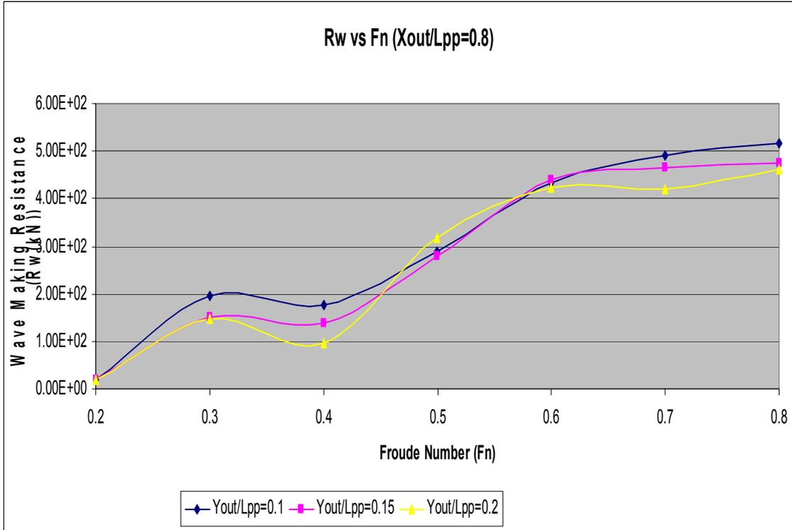
Figure 23. Wave Making Resistance Results for  $X_{out} / L_{pp} = 0.8$
