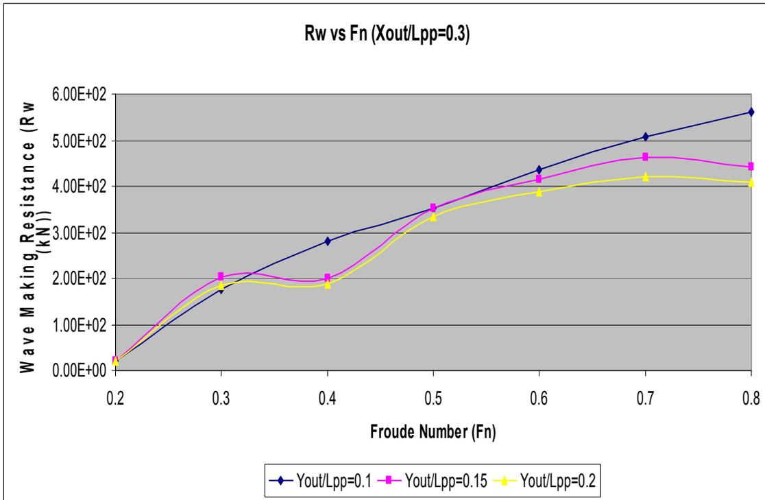
Figure 13. Wave Making Resistance Results for  $X_{out} / L_{pp} = 0.3$
