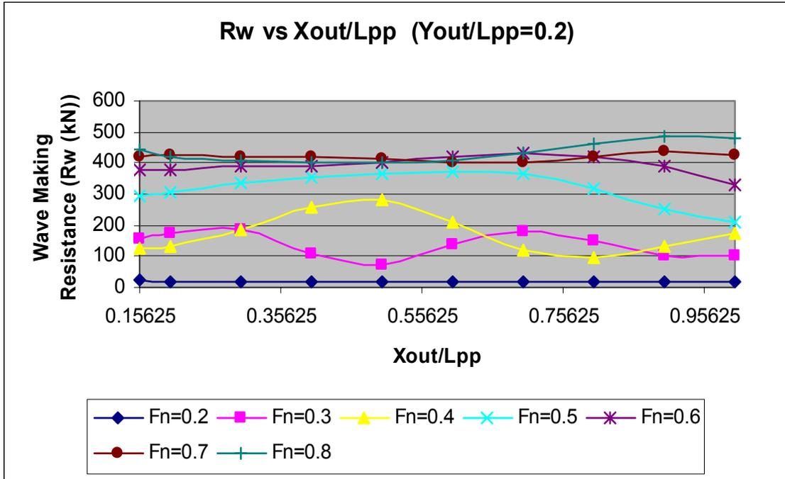
Figure 60. Wave Making Resistance Results for  $Y_{out} / L_{pp} = 0.2$
