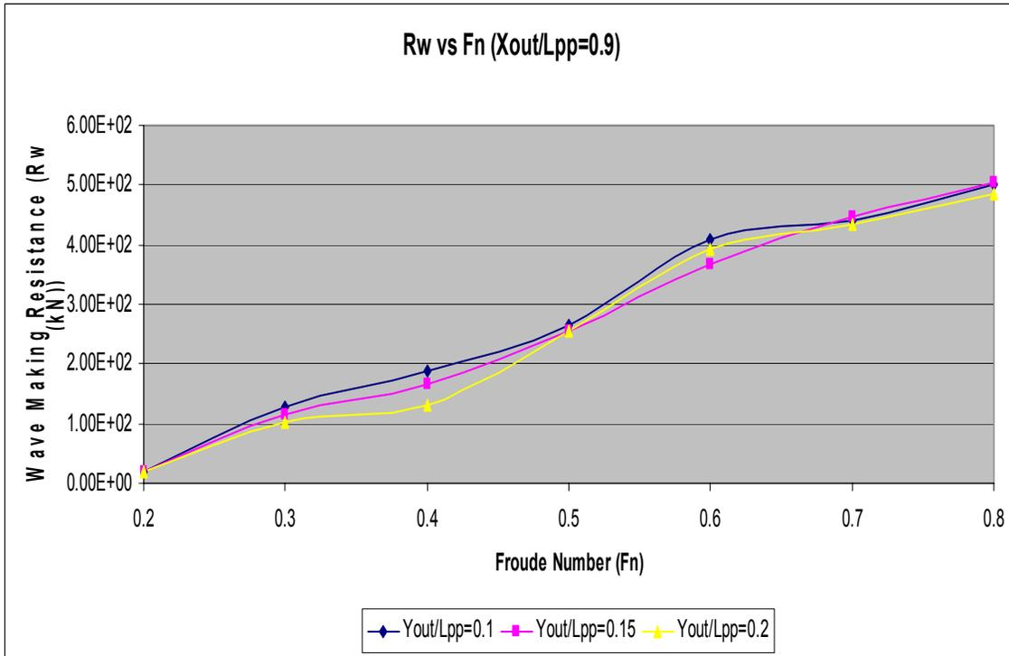
Figure 25. Wave Making Resistance Results for  $X_{out} / L_{pp} = 0.9$
