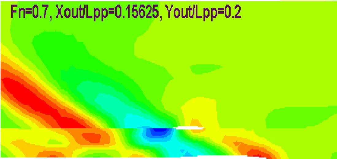
Figure 49. Wave Pattern for  $X_{out} / L_{pp} = 0.15625$  , at Froude Number 0.7
