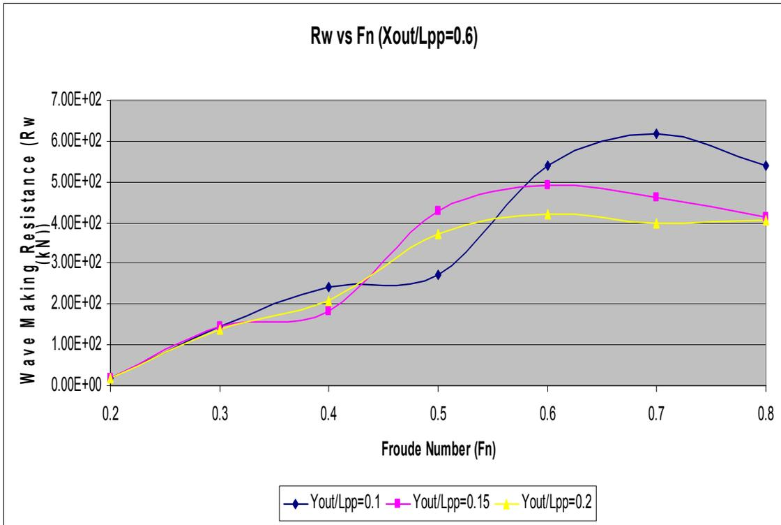
Figure 19. Wave Making Resistance Results for  $X_{out} / L_{pp} = 0.6$
