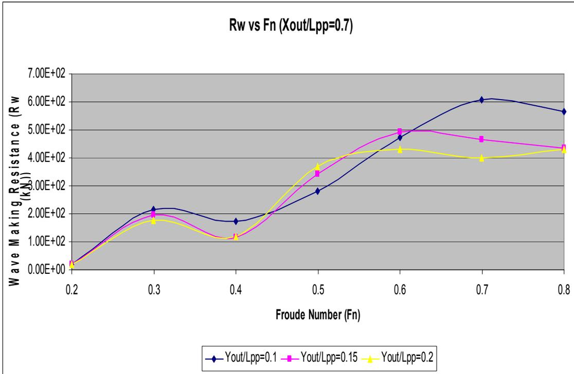
Figure 21. Wave Making Resistance Results for  $X_{out} / L_{pp} = 0.7$
