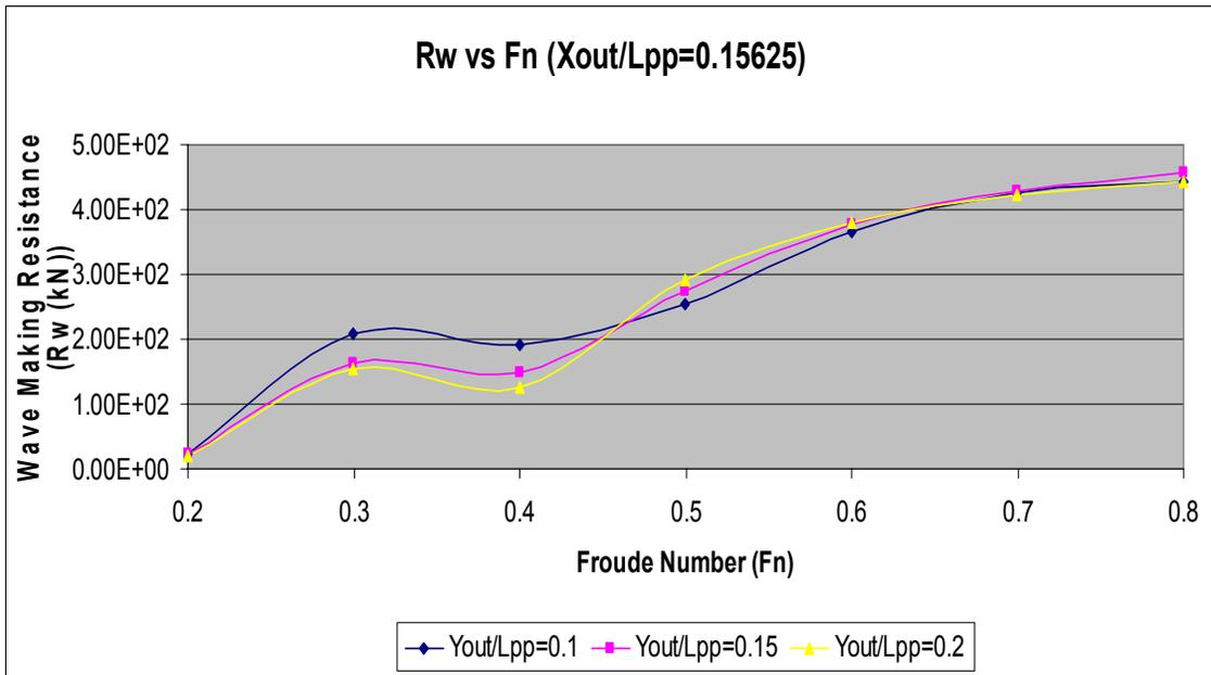
Figure 9. Wave Making Resistance Results for  $X_{out} / L_{pp} = 0.15625$
