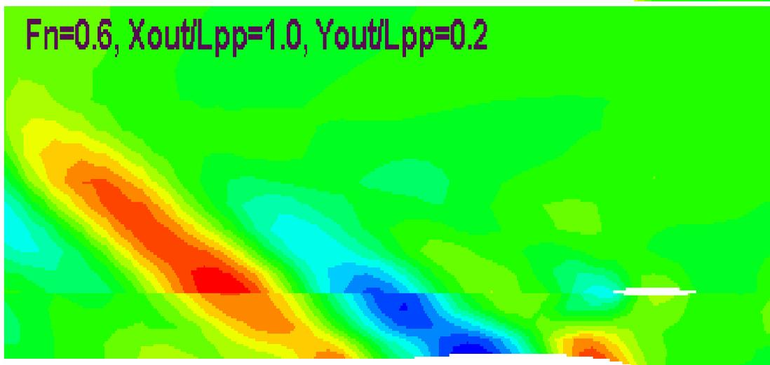
Figure 48. Wave Pattern for  $X_{out}/L_{pp} = 1.0$ , at Froude Number 0.6
