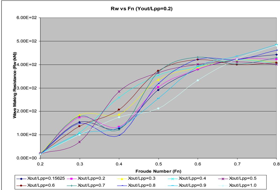
Figure 33. Wave Making Resistance Results for  $Y_{out} / L_{pp} = 0.2$
