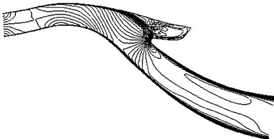
**Fig. 2. Mach number isolines for cruise conditions.**
