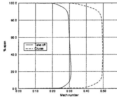
**Fig. 3. Mach number distribution at compressor inlet plane**
