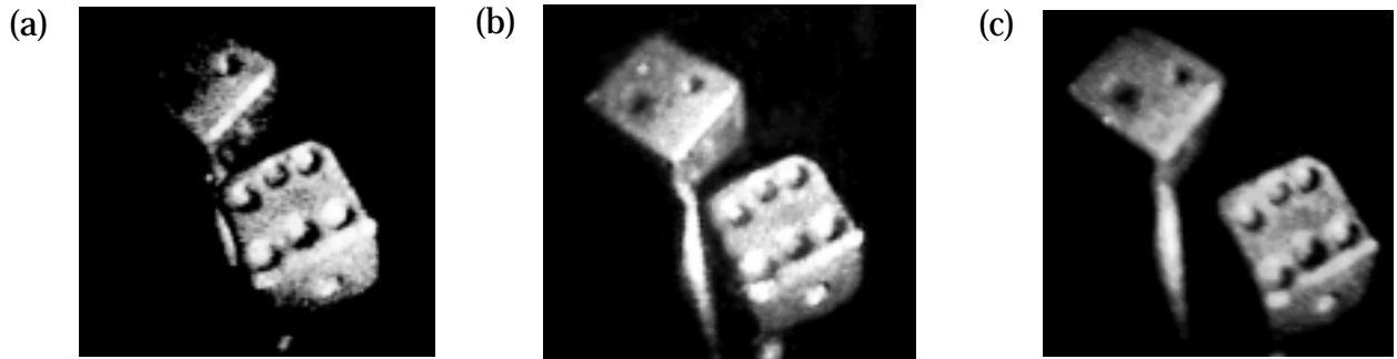
Figure 3. 3-D hologram stored in a Ce-doped SBN:60 photorefractive crystal and viewed at various angles with an FOV of \sim 14^\circ .
