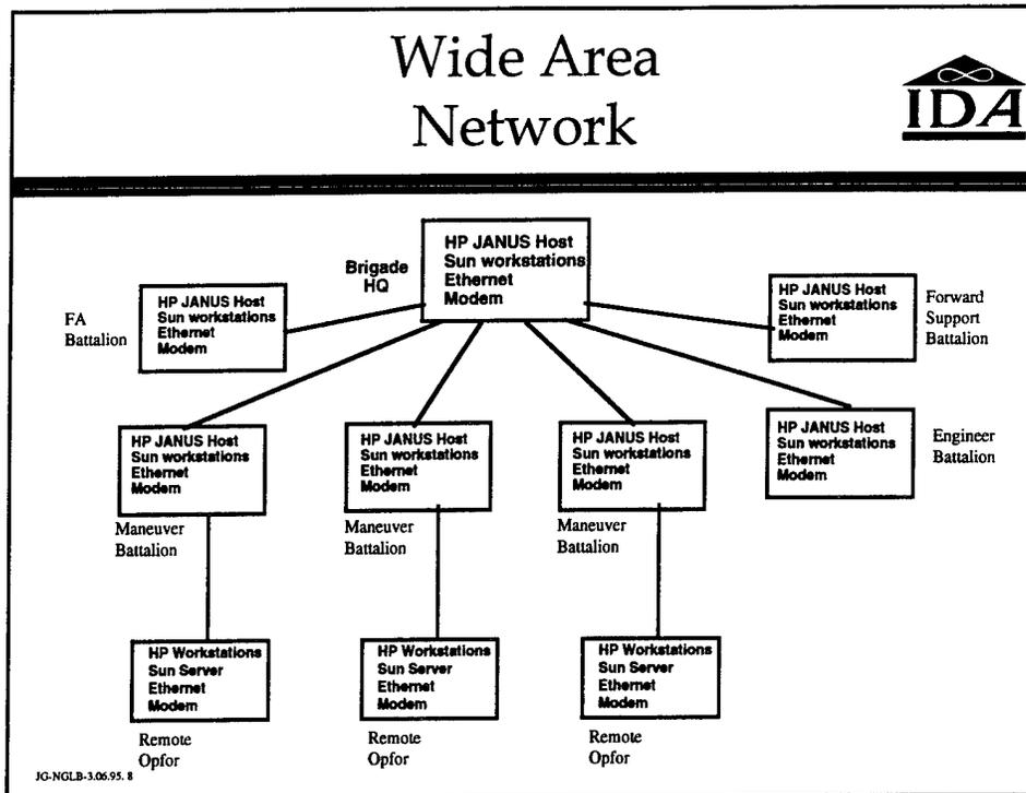
A brigade's subordinate battalions' local-area networks are connected to each other through a star-shaped wide-area network with the brigade server providing connection to all the sites. Each connection includes one data line and four voice lines. The data lines are currently commercial telephone lines, with the servers communicating over 14,400 bps modems using PPP protocols.
