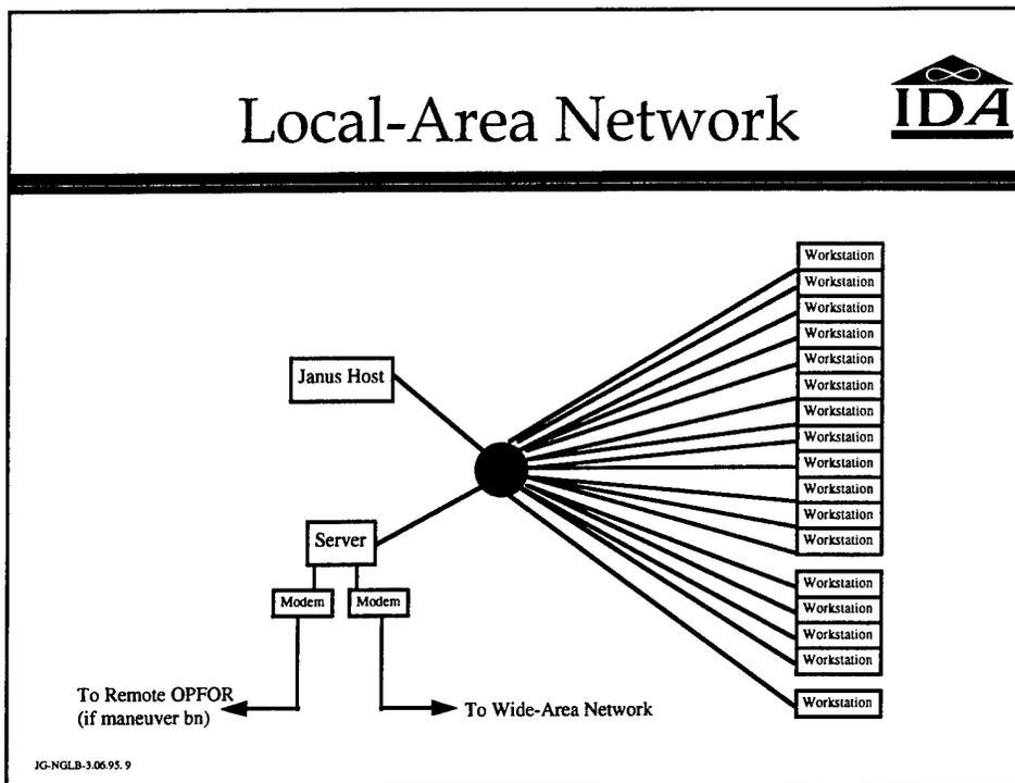
At each unit armory, the local-area network is an ethernet operating off a central set of ethernet hubs. The number of workstations connected to the hub is determined by the requirements of the training exercise. Also connected to the hubs is the Janus host and the Sun server.
