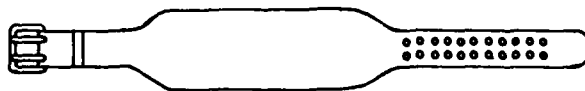
Figure 2—The weight lifting belt drawn to scale. Fabricated of 0.6 cm thick leather, it was 108 cm long, 15 cm wide in its center section, and 6.2 cm wide in its end sections. The belt was worn with its buckle centered over the navel.
