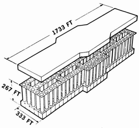
Figure 1. Modular Floating Stable Platform concept.
