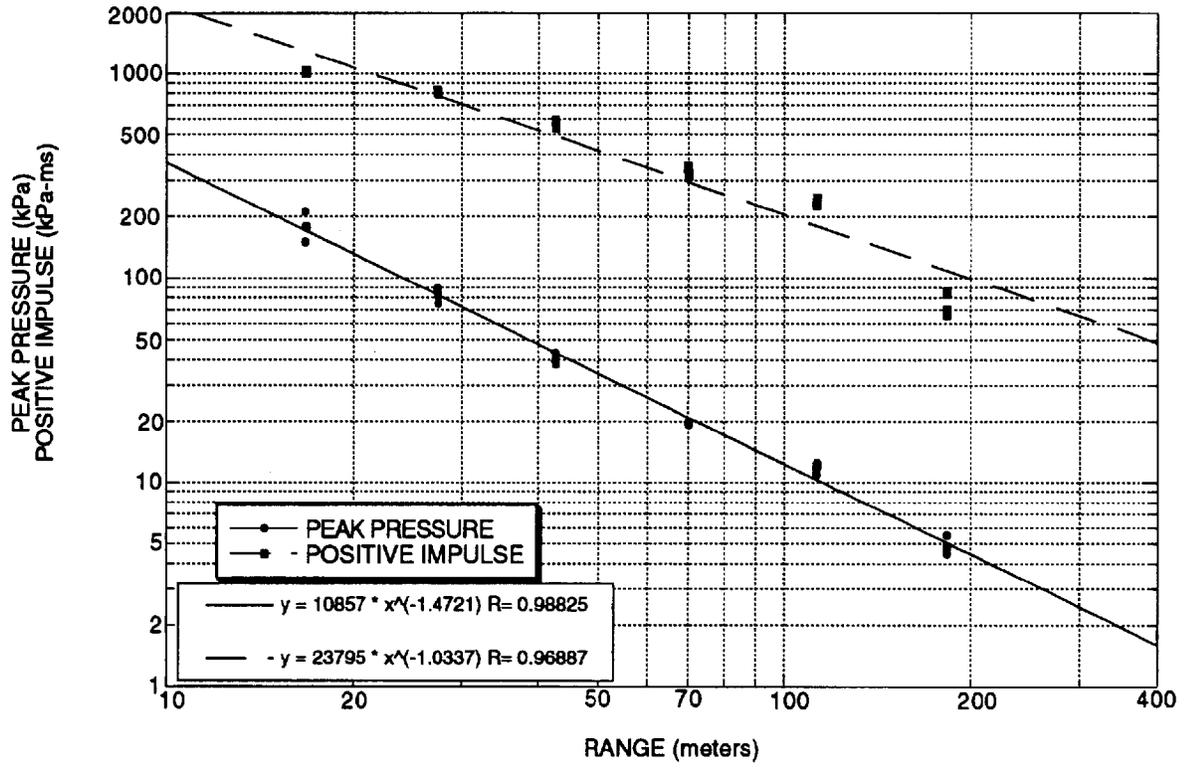
FIGURE 11. CONFIGURATION 6 - AIRBLAST
