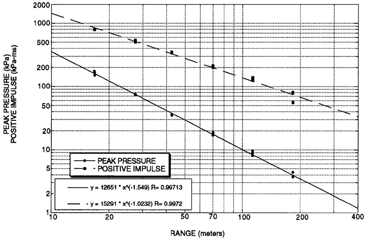
FIGURE 9. CONFIGURATION 4 - AIRBLAST
