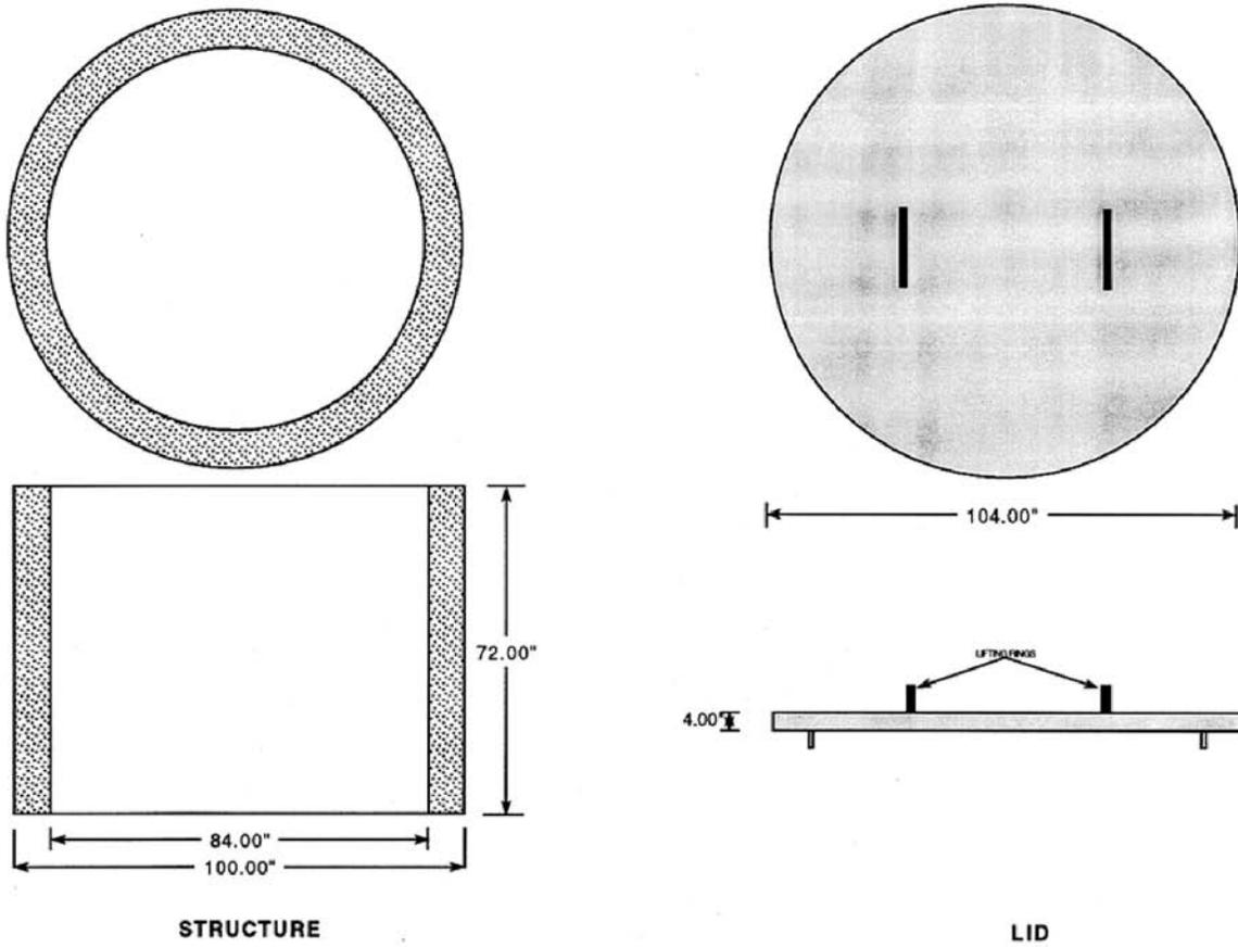
**FIGURE 1. CONTAINMENT STRUCTURE**
