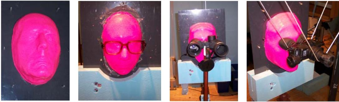
Figure 4. Phantom face model with various eyewear
