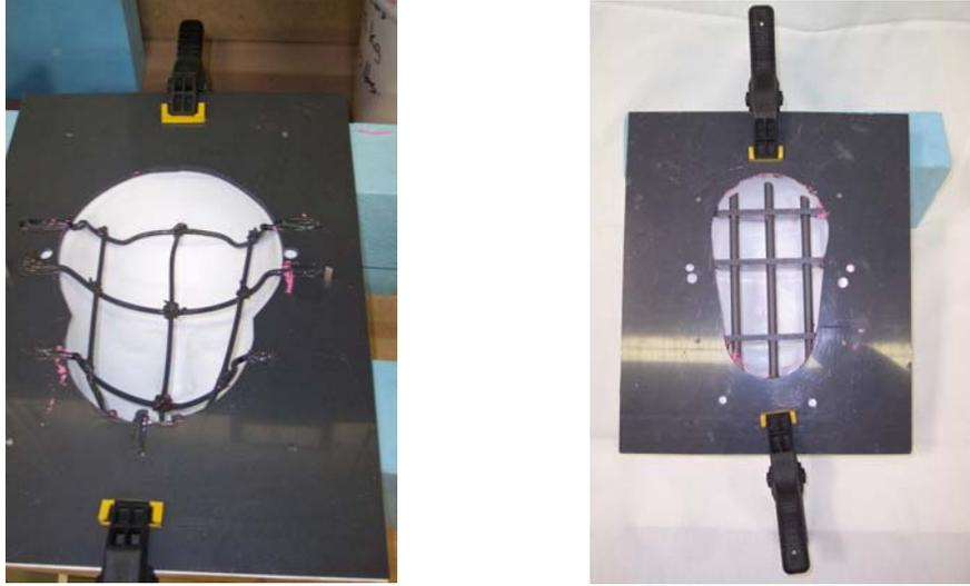
**Figure 3. Mask form holder constructed from PVC**
