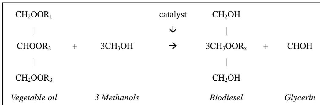
**Figure 3. Biodiesel production.**
