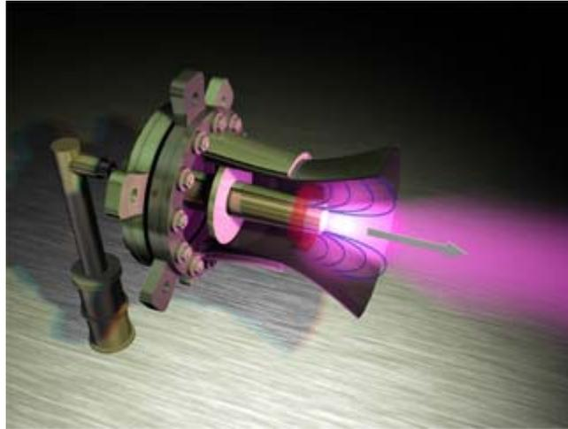
Figure 14: Self-field MPD Thruster
