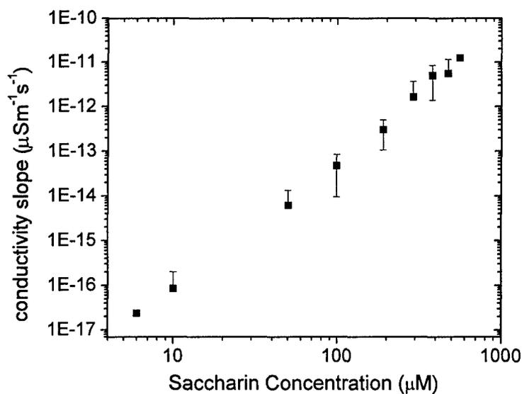
**Figure 17.** Response of nanohybrid sensor to saccharin
