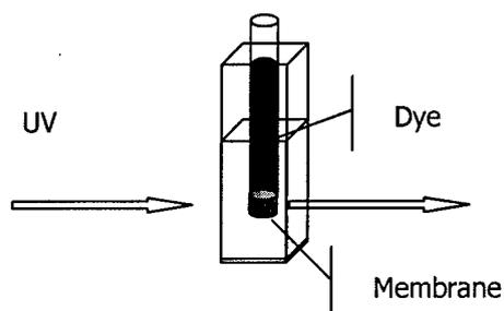
**Figure 10.** Experimental setup used for the permeation experiments
