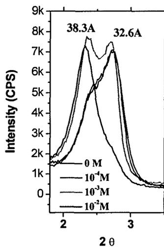
**Figure 18.** X-Ray diffraction patterns of nanohybrids exposed to progressively increasing concentrations of saccharin showing an increase in the gallery height from the original spacing attributed to intercalation of water molecules.
