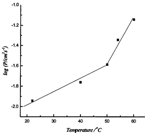
**Figure 13.** Permeability of FH-based nanohybrid at different temperatures
