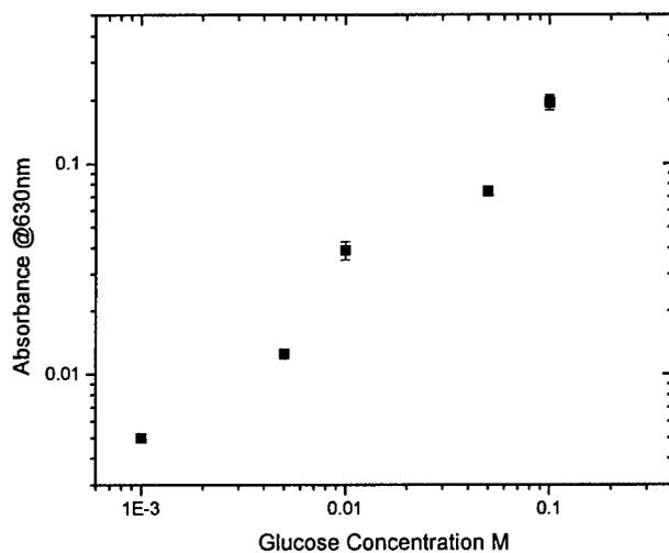
**Figure 20.** Response of Glucose Oxidase Nanohybrid sensor
