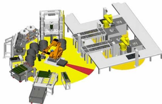
**Automated ADAM Projectile Disassembly Workcell**
